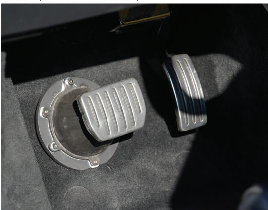
"Instead of using physical connections, the Brake Control Pad senses and sends braking commands electronically, driving towards more precise braking through improved integration with electrification and other advanced driver assistance systems," the release says.
